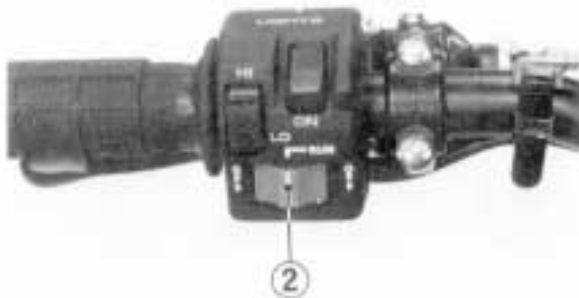
(2) Engine stop switch
