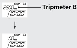
Also, the tripmeter A, average fuel mileage, and fuel consumption will automatically reset by refuelling more than the reserve amount and riding your motorcycle for 0.1 km (0.06 mile).
