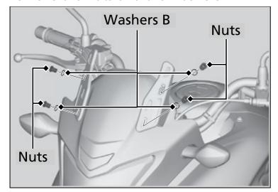
**4.** Set the all nuts and the washers B to the low position holes or high position holes.
