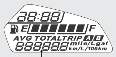
Odometer [TOTAL] & Tripmeter [A/B] & Fuel mileage meter & Fuel consumption meter The SEL button selects the odometer, tripmeter A, tripmeter B, current fuel mileage, average fuel mileage and fuel consumption.
