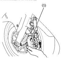
2. Move the left caliper assembly (1) upward while slowly rotating the rear wheel. The brake system is normal if the rear wheel stops. If the rear wheel does not stop, see your Honda dealer.
