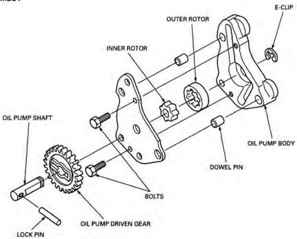
Install the oil pump shaft lock pin into the oil pump shaft. Install the oil pump shaft into the oil pump driven gear.
