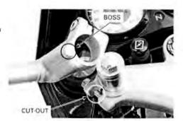
Tighten the handlebar pinch bolt to the specified torque.
