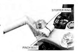
If the left handlebar grips were removed, apply Honda Bond A or its equivalent to the inside surface of the grip and to the clean surface of the left handlebar. Wait 3 - 5 minutes and install the grip.
