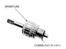
Check for continuity between pairs of commutator bars. There should be continuity.
