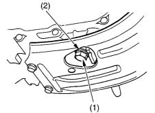
(1) oil drain bolt(2) sealing washer
