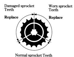
If the drive chain or sprockets are excessively worn or damaged, they should be replaced. Never use a new chain with worn sprockets; rapid chain wear will result.
