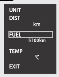
To end the each meter unit setting, select "EXIT" menu, and then the display returns to the main menu screen.
