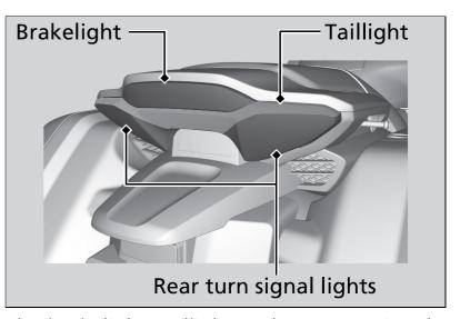
The brakelight, taillight and rear turn signal lights use several LEDs.
