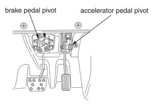
Lubricate the parking brake pivot as shown in the following illustration. Remove the center panel (page 120).
