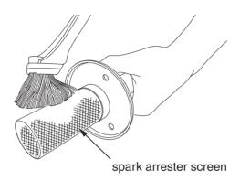
4. Install the spark arrester and the gasket in the muffler, and tighten the bolts to the specified torque:
