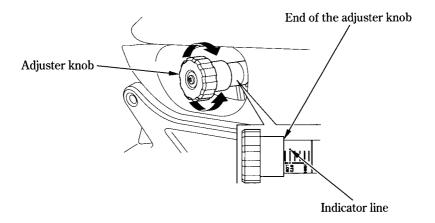
The rear shock absorber assembly includes a damper unit that contains high pressure nitrogen gas. Do not attempt to disassemble or service the damper; it cannot be rebuilt and must be replaced when worn out. Disposal should only be done by your Honda dealer. The instructions found in this owner's manual are limited to adjustment of the shock assembly only.
