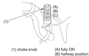
1. If the engine is cold, pull the choke knob (1) up all the way to fully ON (A) position.
