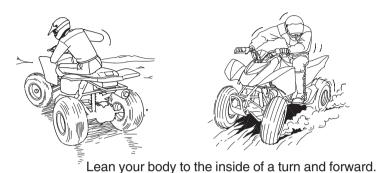
To make a turn on level ground: Steer the handlebar and lean your body
