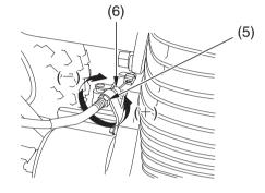
(5) lower adjusting nut(6) lower lock nut
