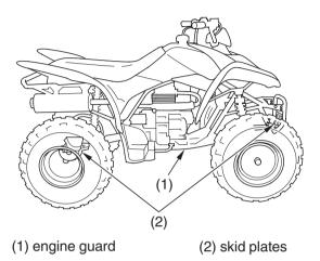
The engine guard (1) protects the engine crankcase.
