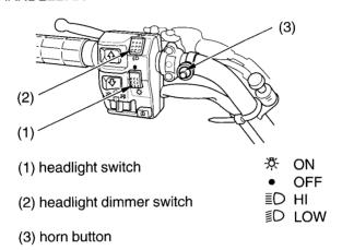
The headlight switch (1) is used to turn the headlight ON ( $\clubsuit$ ) or OFF ( $\bullet$ ). To operate, turn the switch to ON ( $\clubsuit$ ) or OFF ( $\bullet$ ).
