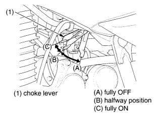
The choke lever may be used when starting the engine. See page 44.
