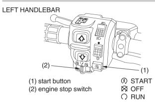
The start button (1) is used for starting the engine. Pushing the button in starts the engine. See *Starting Procedure*, page 64.
