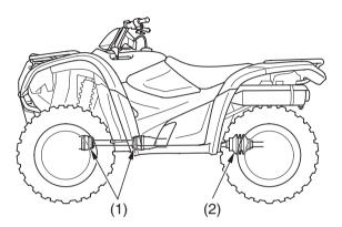
(1) rubber propeller shaft boots (Except TRX420TE)(2) rubber yoke joint boot
