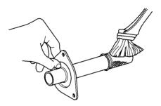
4. Install the gasket to the muffler, the spark arrester, and the muffler tail cover and tighten the three bolts securely.
