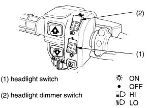
The headlight switch (1) is used to turn the headlight ON (♣) or OFF (•). To operate, turn the switch to ON (♣) or OFF (•).
