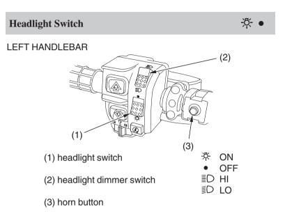
The headlight switch (1) is used to turn the headlight ON (  $\$  ) or OFF (  $\$  ). To operate, turn the switch to ON (  $\$  ) or OFF (  $\$  ).
