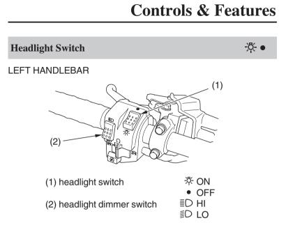
The headlight switch (1) is used to turn the headlight ON (  $\stackrel{\infty}{\rightarrow}$  ) or OFF ( • ). To operate, turn the switch to ON (  $\stackrel{\infty}{\rightarrow}$  ) or OFF ( • ).
