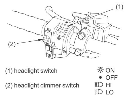
The headlight switch (1) is used to turn the headlight ON ( $\ \ \ \ \ \ \ \ \ \$ ) or OFF (  $\ \ \ \ \$ ) or OFF (  $\ \ \ \ \$ ).
