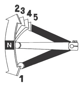
The shift lever is located near the left footpeg. One full stroke of the shift lever shifts the transmission to the next higher or lower gear in the shifting sequence. The shift lever automatically returns to the horizontal position when released.
