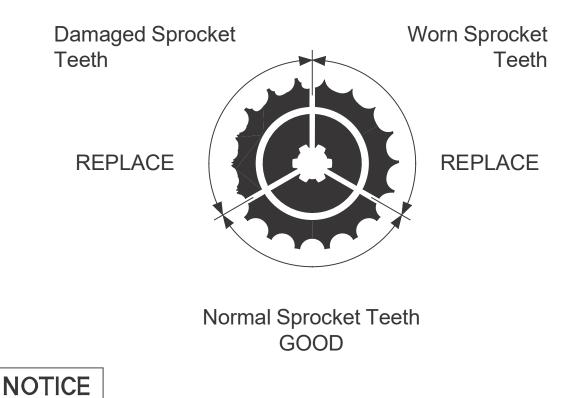
Use of a new chain with worn sprockets will cause rapid chain wear.
