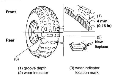
To check the condition of a tyre tread, measure the groove depth (1) in the centre of the tyre, or check the wear indicator (2).
