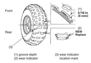
To check the condition of a tire tread, measure the groove depth (1) in the center of the tire, or check the wear indicator (2).
