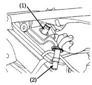
(1) Spark plug wrench (2) Spark plug cap
