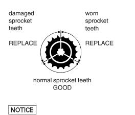
Use of a new chain with worn sprockets will cause rapid chain wear.
