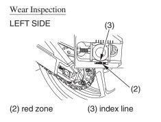
Check the chain wear label when adjusting the chain. If the red zone (2) on the label aligns with the index line (3) on the chain adjuster plates after the chain has been adjusted to the proper slack, the chain is excessively worn and must be replaced. The proper slack is: 1-1 3/8 in (25-35 mm)
