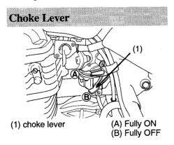
The choke lever, used for starting the engine (page 30), increases the percentage of fuel in the fuel/air mixture delivered to the engine.
