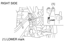
With the motorcycle in an upright position, check the fluid level.
