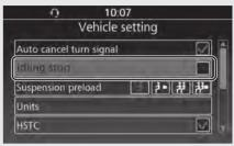
Select [Idling stop], and then press or ENT switch to change to select (enable) or deselect (disable) the function.
