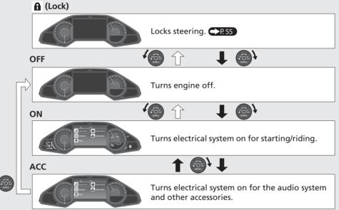
: Turning the ignition switch clockwise.
