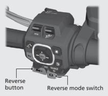
When you are ready to back up, press and hold the Reverse button. The motorcycle will move in reverse as long as you hold the button down. ("R" is displayed on the gear position indicator.)
