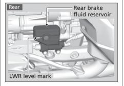
If the brake fluid level in either reservoir is below the LWR mark or the brake lever and pedal freeplay becomes excessive, inspect the brake pads for wear. If the brake pads are not worn, you most likely have a leak. Have your motorcycle inspected by your dealer.
