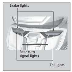
The brake lights, taillights and rear turn signal lights use several LEDs. If there is an LED which is not turned on, see your dealer for servicing.
