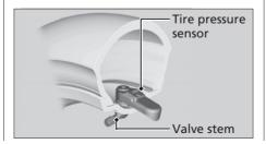
Each tire has its own pressure sensor. If the air pressure of a tire becomes significantly low while riding, the sensor in that tire sends a signal that causes the low tire pressure indicator to turn on.
