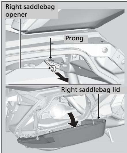
5. Install the right saddlebag opener onto the prong before closing the saddlebags.
