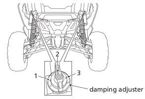
The damping adjuster has 3 positions for different load or driving conditions.
