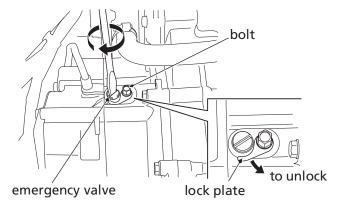
3. Return the lock plate and tighten the bolt securely.
