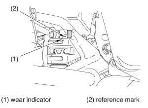
Check the wear indicator. If the wear indicator (1) aligns with the reference mark (2), replace both pads as a set, see your dealer for this replacement.
