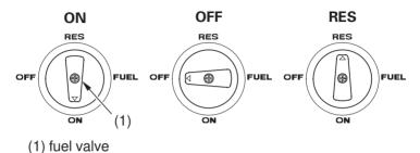
The manual fuel valve (1) is located on the left side of the fuel tank cover.
