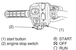
The start button (1) is used for starting the engine. Pushing the button in starts the engine. See *Starting Procedure*, page 69.
