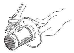
4. Install the spark arrester and gasket in the muffler, and tighten the bolts to the specified torque:
